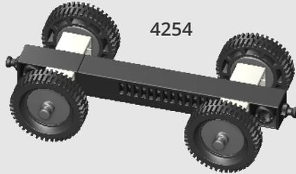
**4.** For **case 3** reverse each pulley and put it back to the model. This way the rounded connection of the pulley is connected on the model instead of the octagon one and the wheels are free to rotate. Repeat the procedure of **step 2** and do **exercises 4** and **5**.
